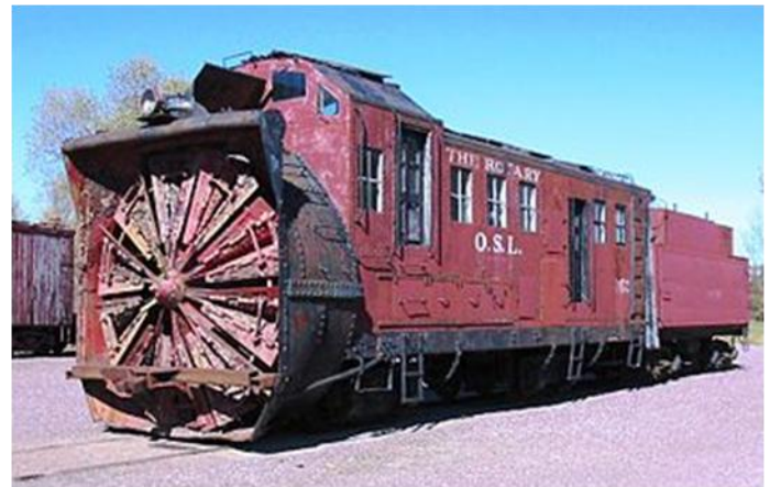
A rotary snowplow from the Oregon Short Line on display at the Mid- Continent Railway Museum in North Freedom, WI
