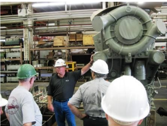
Part of the shop tour. NWHS members were escorted through Roanoke's famous East End Shops where NS overhauls GE locomotives. Here we see the general foreman with a new 4400 HP prime mover for a GE D-9 40CW locomotive. NS is very restrictive on visitation; getting inside of these facilities is quite a privilege.
